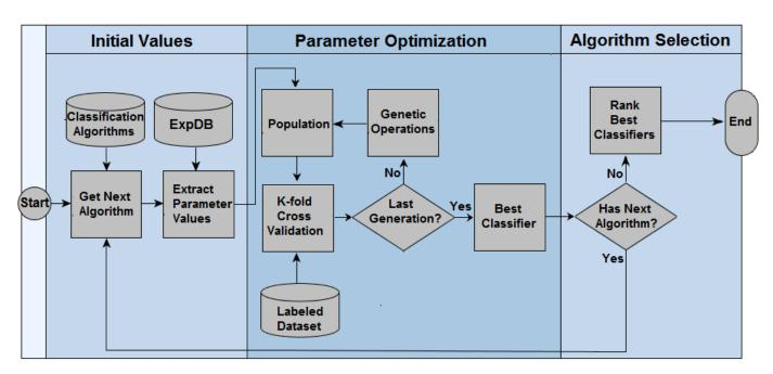
Fig. 1. Methodology for parameter optimization and algorithm selection.
