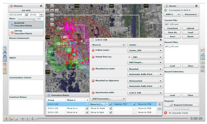
Fig. 2. GMI: Entering detailed Mission Order in Execution Matrix format modeled after US Army standard.
