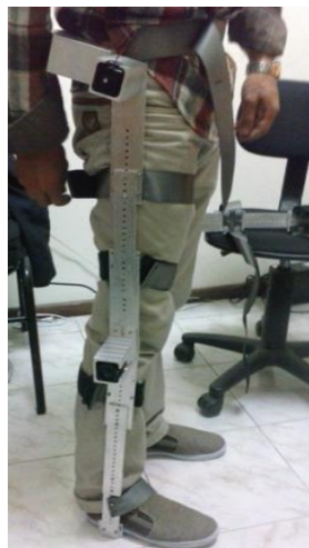
Fig.2 Represents the Exoskeleton that it was built and where the control tests were performed.
