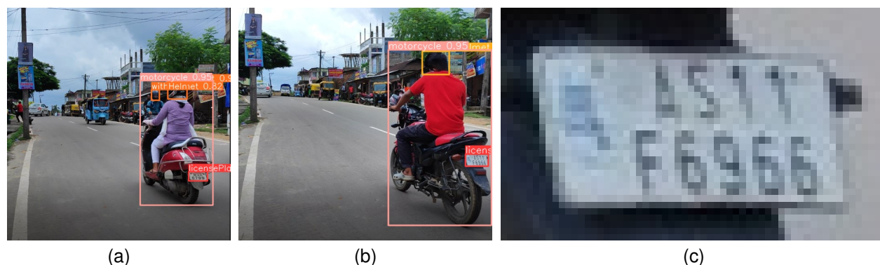
Fig. 6. Inferences from the model. (a) A biker with Helmet. (b) A Biker without Helmet. (c) Extracted Numberplate. Here (c) is the numberplate extracted from (b), i.e. without helmet biker
