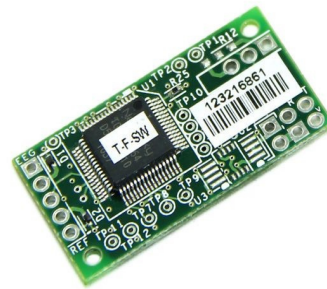
Fig. 2. Sensor ThinkGear ASIC Module v1.0 (TGAM1)
