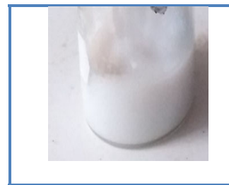
Fig. 1. Nanoparticles coated with Polysorbate 80 as passivating agent
