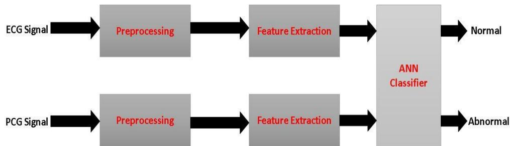
**Fig. 1.** The block diagram for cardiac monitoring using PCG and ECG recording
