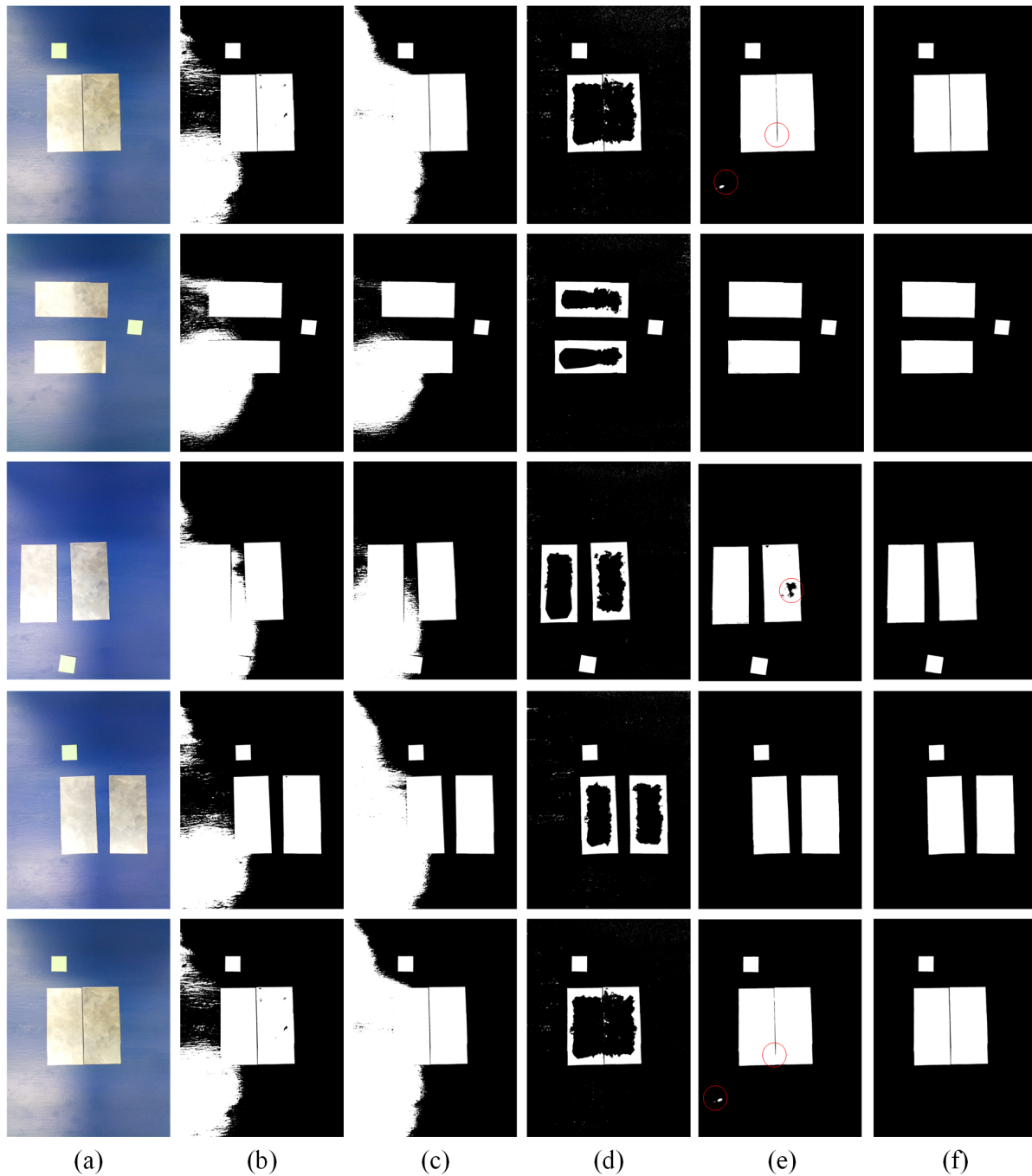
Fig. 5. Comparison of binaries images results of different algorithms. (a) Input image, (b) Entropy thresholding, (c) Otsu algorithm, (d) Adaptive thresholding, (e) HSV binarization, (f) Proposed algorithm binarization
