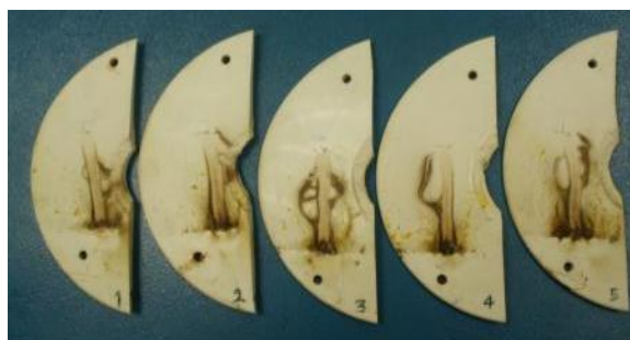
Fig. 6. Specimens evaluated in inclined plane test, Brand I
