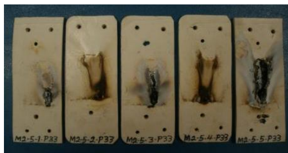
Fig. 5. Conventional shape of the specimens tested in IPT
