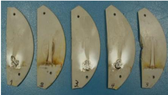
Fig. 7. Specimens of Brand II after evaluation in IPT
