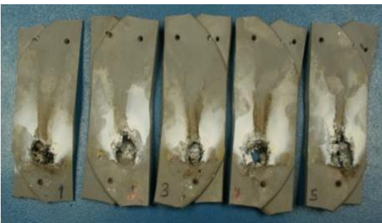
Fig. 9. Specimens of Brand III after evaluation in IPT (double shed)
