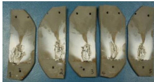
Fig. 11. Specimens of Brand V after evaluation in IPT
