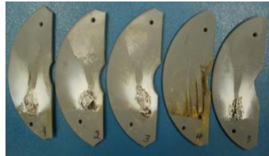
Fig. 10. Specimens of Brand IV after evaluation in IPT
