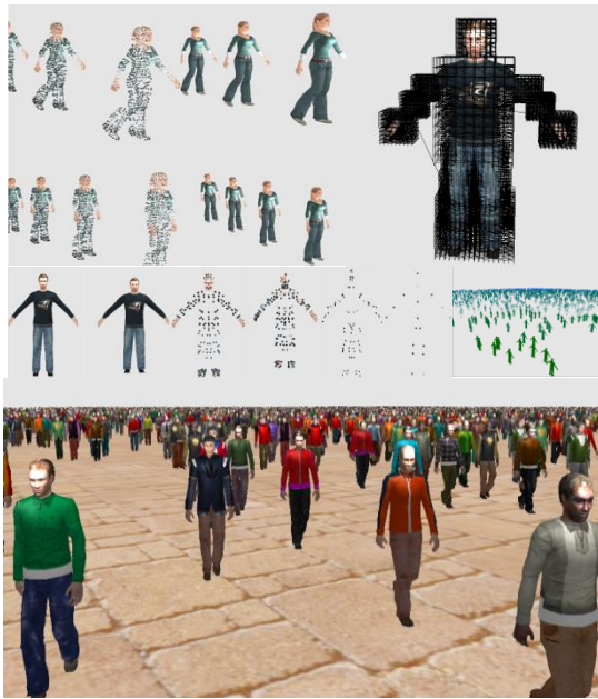
Fig. 13. Point rendering vs geometric models (top left). Hierarchical skeleton structure based on octrees (top right). Different Levels of Detail and coding (middle). Scene rendered using complete system (bottom)
