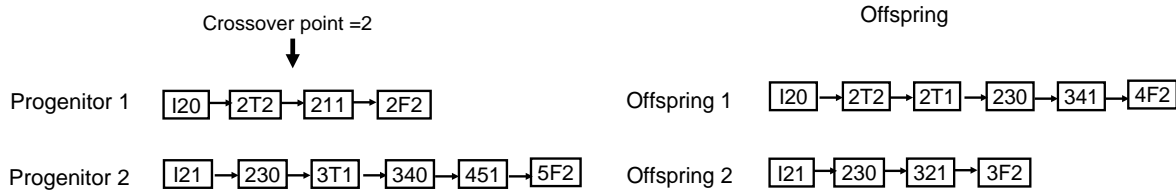
Fig. 7. An example illustrating the crossover operator
