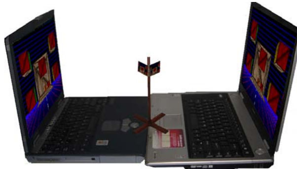
Fig. 4. Wheatstone-Mora environment built with two monitors
