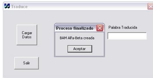
Fig. 6. The Alpha-Beta Bidirectional Associative Memory is built by associating 120 words in Spanish with 120 words in English, which are contained in two text files.
