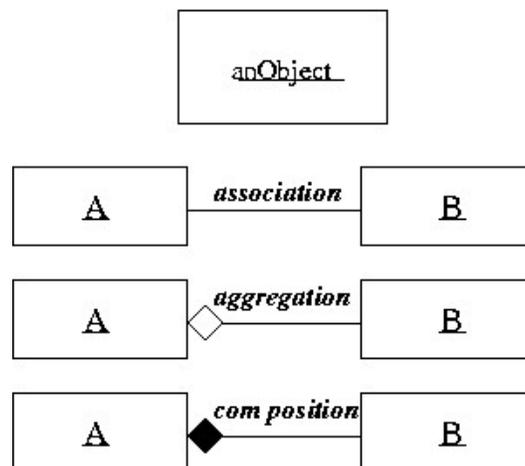
**Fig. 1.** Basic elements of an Object Diagram
