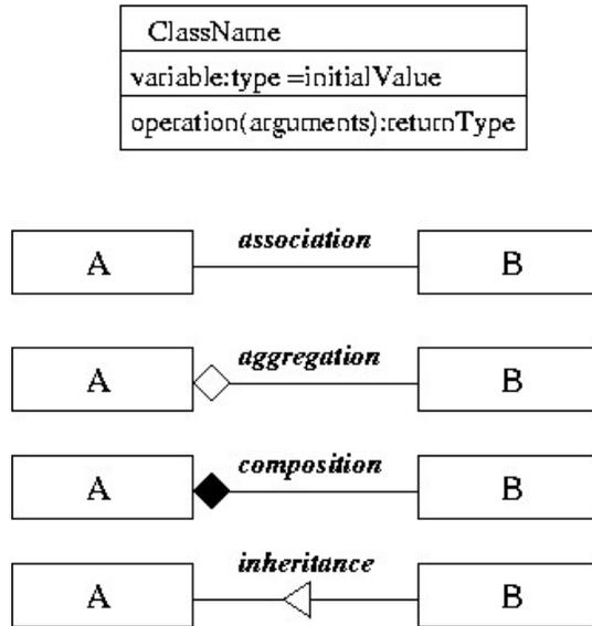
Fig. 2. Basic elements of a Class Diagram
