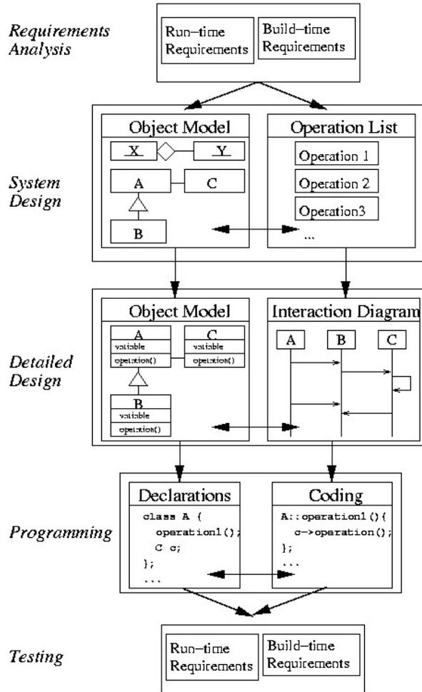
Fig. 4. Phases of the Practical Design Method
