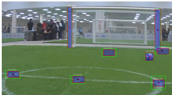
Fig. 3. Example of detected landmarks with the Deformable-DETR model
