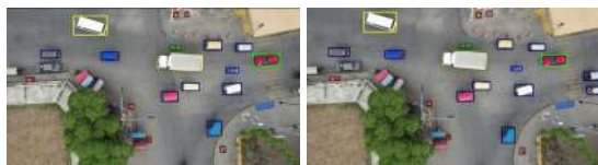
Fig. 4. Object detection with YOLOv4 at two different frames of the video
