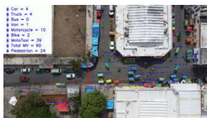
Fig. 6. Automatic counting system at a given frame of the video 0362
