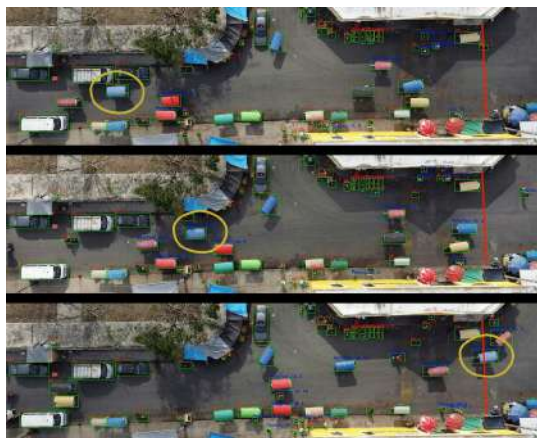
Fig. 5. Object tracking based on the IoU metric. The red segment indicates the region of interest provided by the user where crossing objects are counted. The tracked object is depicted with a yellow ellipse. From top to bottom: different steps towards the counting of an object
